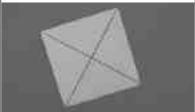
Using diagonals to locate the center of the square wheel
