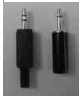
A mono plug (right) has one black band. A stereo plug (left) has two.
