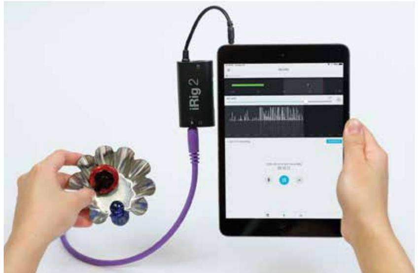
After testing different hardware solutions, we found that a contact microphone with an iPad amplifier and headphones work best for the purpose. Visitors can use this contact mic like a stethoscope to closely listen to otherwise inaudible sounds. We often describe it as a magnifying glass for sound. We observed curiosity and delight as visitors moved around the workshop area on a "Sound Safari" to
