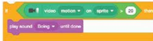
A variable block. The video sensing can detect the amount of the motion on a specific sprite or the entire background.
