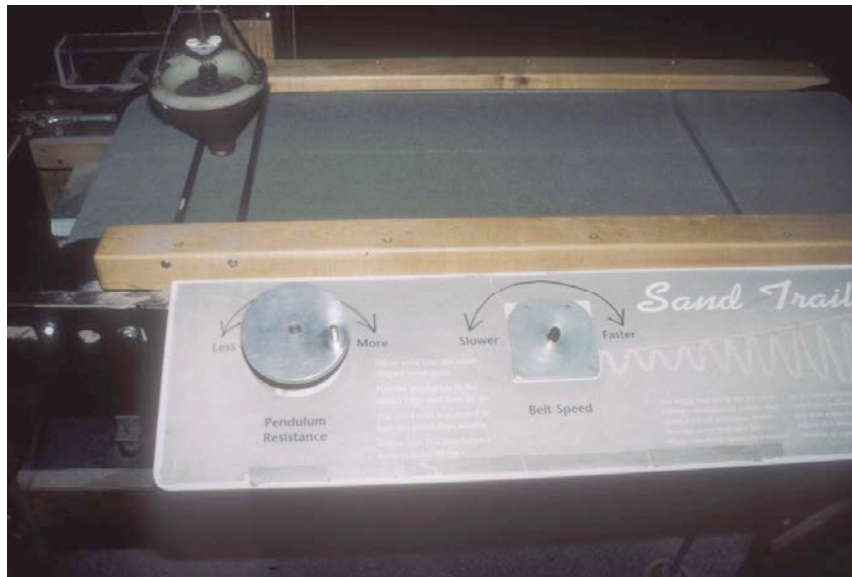
Figure 9. Control knobs on original Fading Motion exhibit (formerly Sand Trail). The large dial on the left controls the damping mechanism, while the small knob on the right control the belt speed. Photo courtesy of the Exploratorium.
