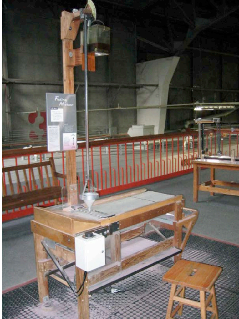
Figure 10. Revamped Fading Motion exhibit, with damping control removed and belt drive control made more salient. Photo courtesy of the Exploratorium.
