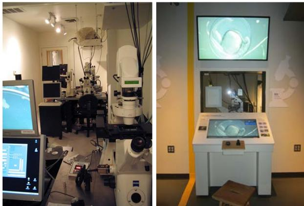
**Figure 1. The Microscope Imaging Station, (left) the equipment inside the biology lab, and (right) the user kiosk.**
