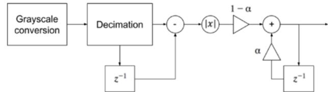
**Figure 3. Heart detection algorithm flowchart.**
