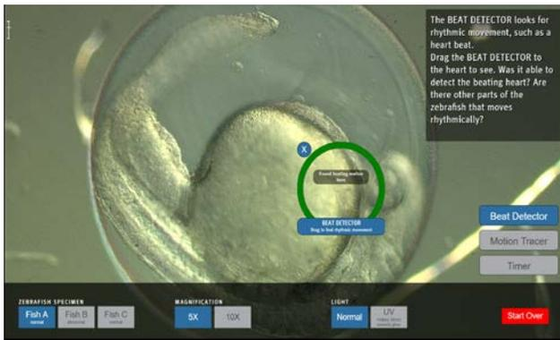
**Figure 5. Technology as tool. The Beat Detector can be dragged over the live image to detect rhythmic movement. Green denotes that the system has detected rhythmic motion within the circle. In this screenshot, the Beat Detector has been dragged over the heart and shows green.**
