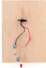
8. Place a washer onto another screw. Wrap the other side of the resistor to the screw. Strip 1/4 inch (6 mm) of insulation off the wire from the negative (black) side of the 9-volt battery connector and wrap it around the screw. Screw it to the board.
