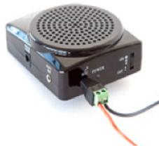
4. To test if the receiver is working, turn on the voice amplifier and place the solar cell under a set of fluorescent lights. Many fluorescent lights flash at about 120 Hz, so you should hear a steady buzz from the speaker. Alternatively, you can shine a flashlight onto the speaker. Flash the light on and off. You should hear a click from the speaker each time the light goes on or off.
