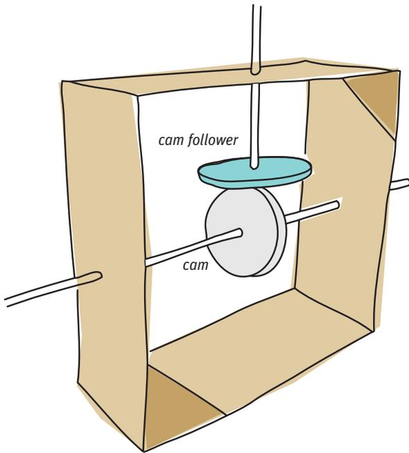
The spinning element that you turn with the handle is called a cam. The element that sits on top of the cam will move according to the shape and position of the cam, and is called a cam follower. The cam follower transmits its motion to the elements on top of the box to animate your sculpture.
