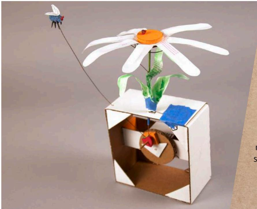
Cardboard automata is a type of mechanical sculpture made of simple materials that lets you bring stories to life. As you build you can explore simple machine elements such as cams, levers, and linkages in a playful way. Making this version of automata lets you quickly get started in building functional mechanisms as your mechanical sculpture ideas develop.
