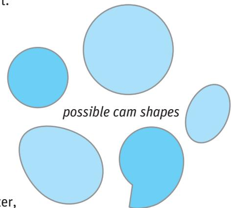
*Tip: Cut the cams smoothly and make sure the cam follower is a little bigger than the cam. As you make more automata, experiment with different shapes and sizes to see how they affect the automata motion.*
