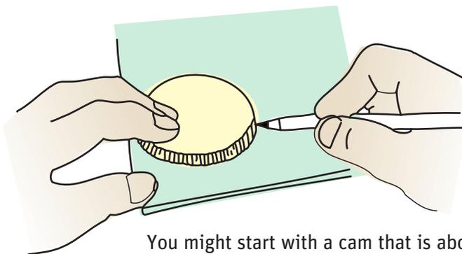
You might start with a cam that is about 2.5" in diameter, then experiment with other sizes based on your design.
